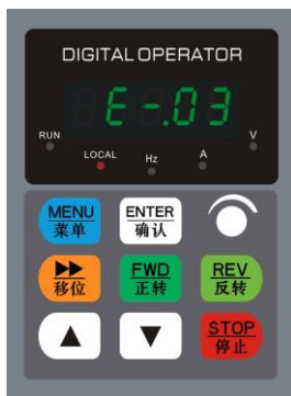
Fig. 4-5 Fault alarm display state
