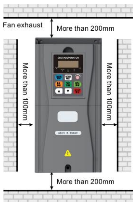
Fig.3-1 Mounting space and distance
