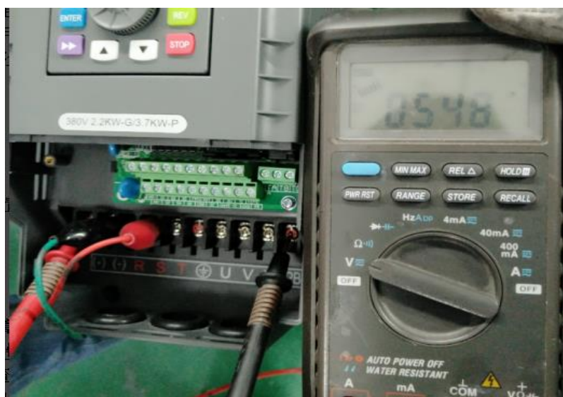
Figure 5 Schematic diagram of brake circuit measurement
