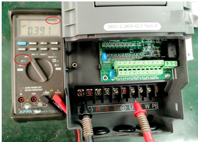
Figure 3. Schematic diagram of three-phase upper bridge measurement in the inverter part
