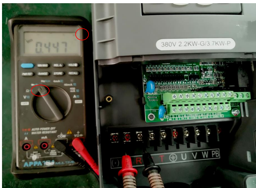
Figure 2. Schematic diagram of three-phase lower bridge measurement in the rectification section
